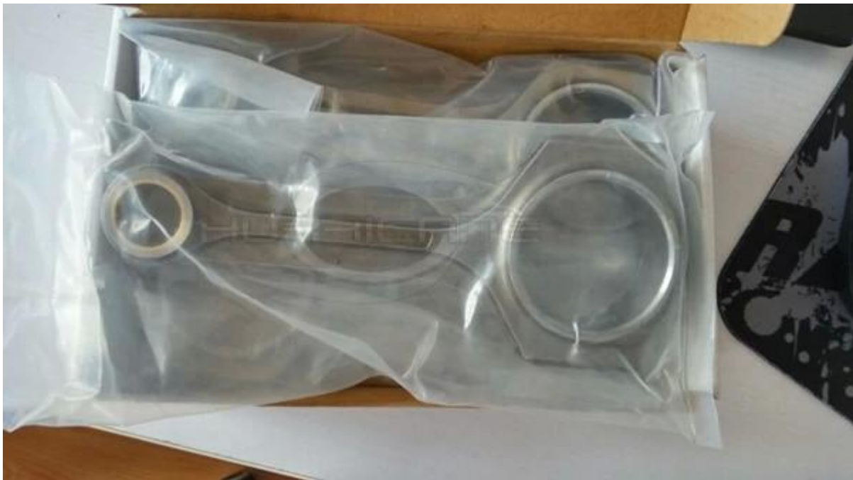
Finished X-beam connecting rods
