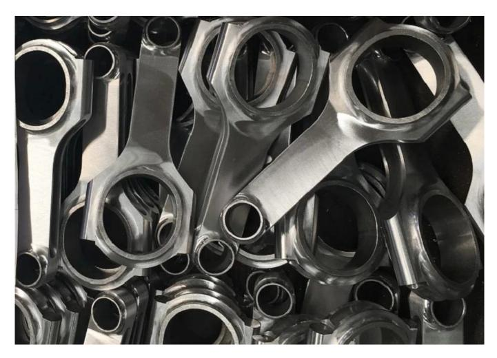
Note: Burring, polishing,(remove burrs and make surface smooth) and shot blasting (Small ball hit surface and make them on surface, increase rods strength with Small ball) are all crucial operations in the making of a competition connecting rod. You can check more detailed information at: <a href="https://document.com/html/>
