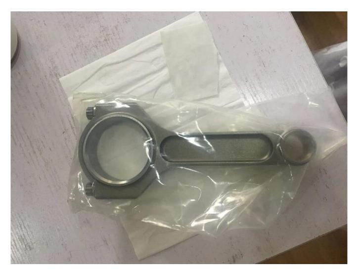
Racing rod for Ford 460 6.605" I-beam are the strongest, advise horsepower 1600HP.
