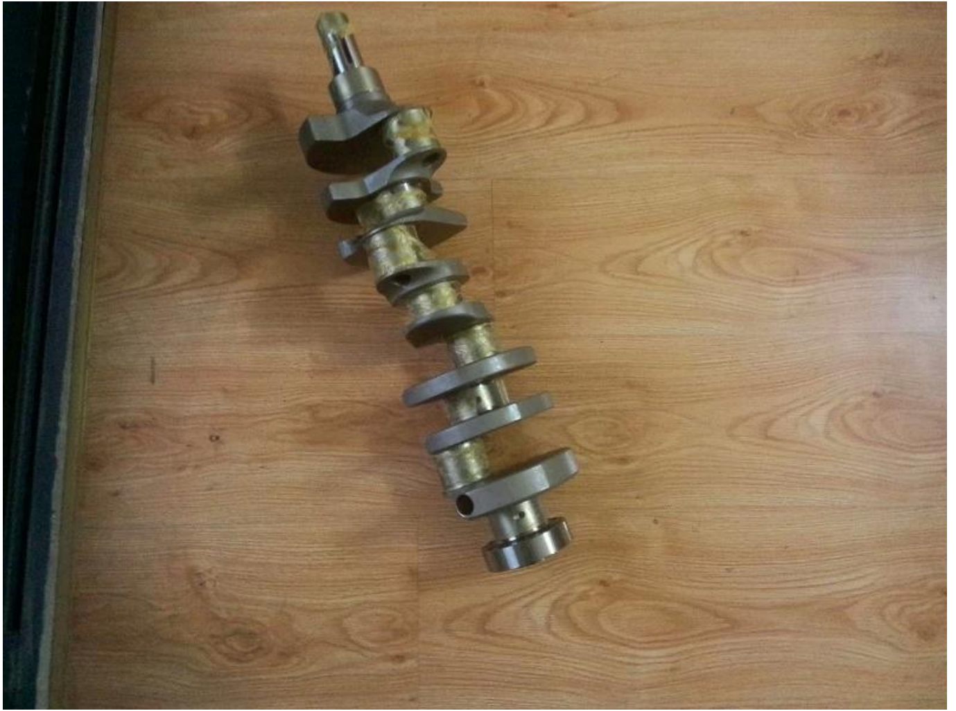
Hurricane Ford Small Block 302 3.250" Cranks Are Magna Fluxed, Shot Peened And All Journals Are Nitrided, Precision Ground And Micro Polished. Those progress will added srength and journal hardness.
