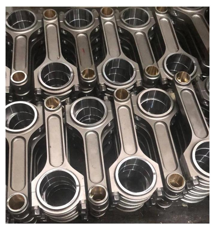
Note: Hurricane I beam connecting rods dodge srt-4 are ready for honing, every piece of Heavy Duty SRT-4 connecting rods will be honed to use size by Sunnen Honing Machine.
